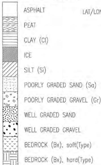
SOFT OR HARD BEDROCK BASED ON DRILLING RATE
