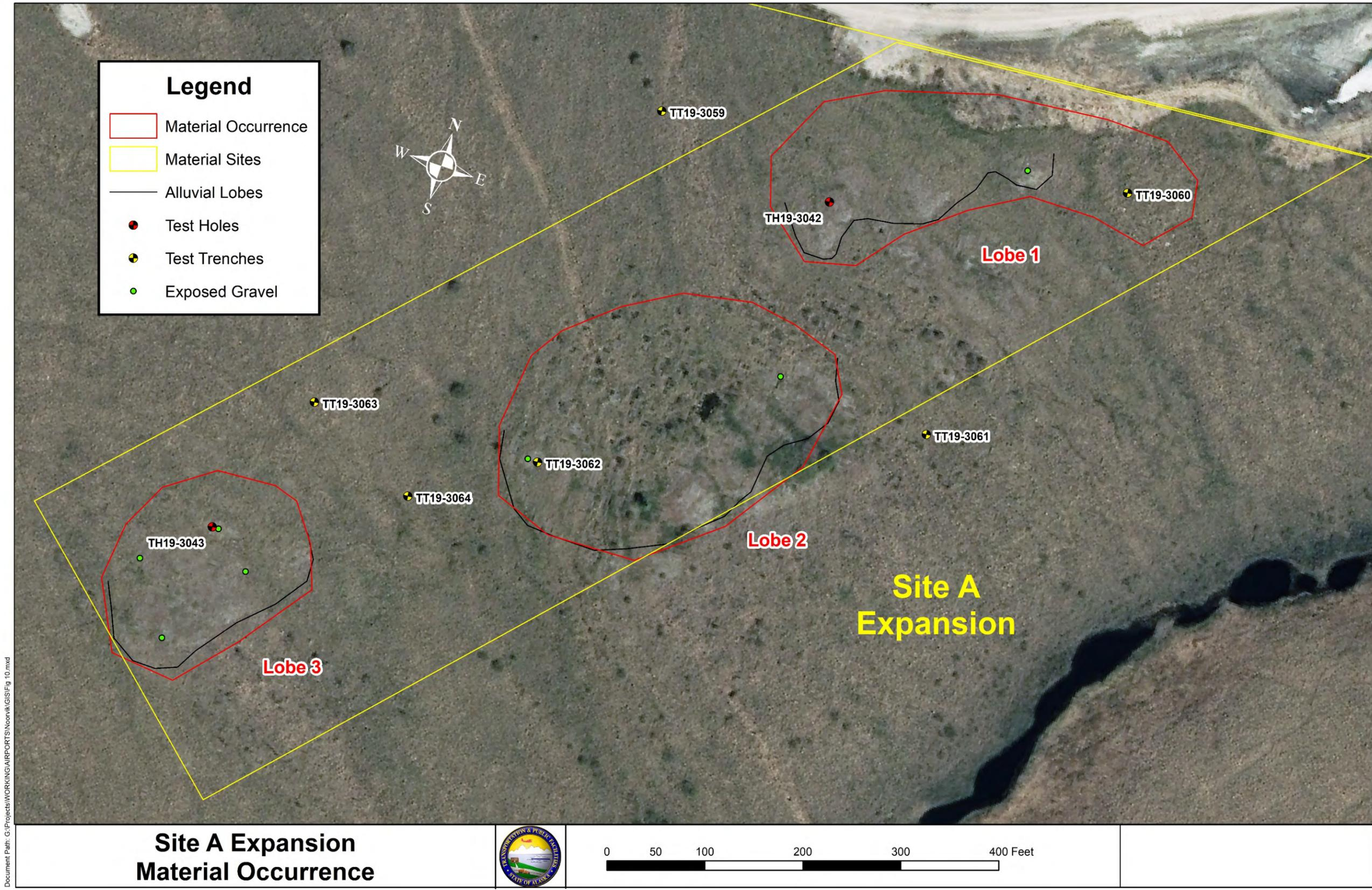
Figure 10. Locations of Site A test drilling and trenching.
