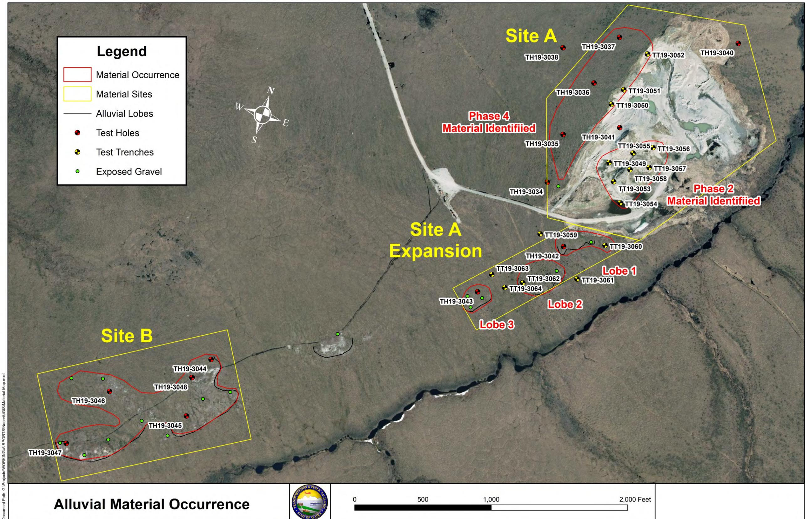
Figure 8. Locations of all material test drilling and trenching.
