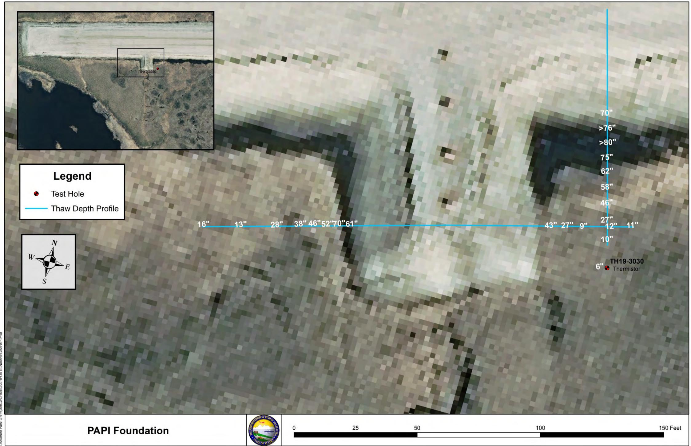
Figure 6. Location of thaw depth profiles adjacent to PAPI showing depth of thaw at intervals along the profile
