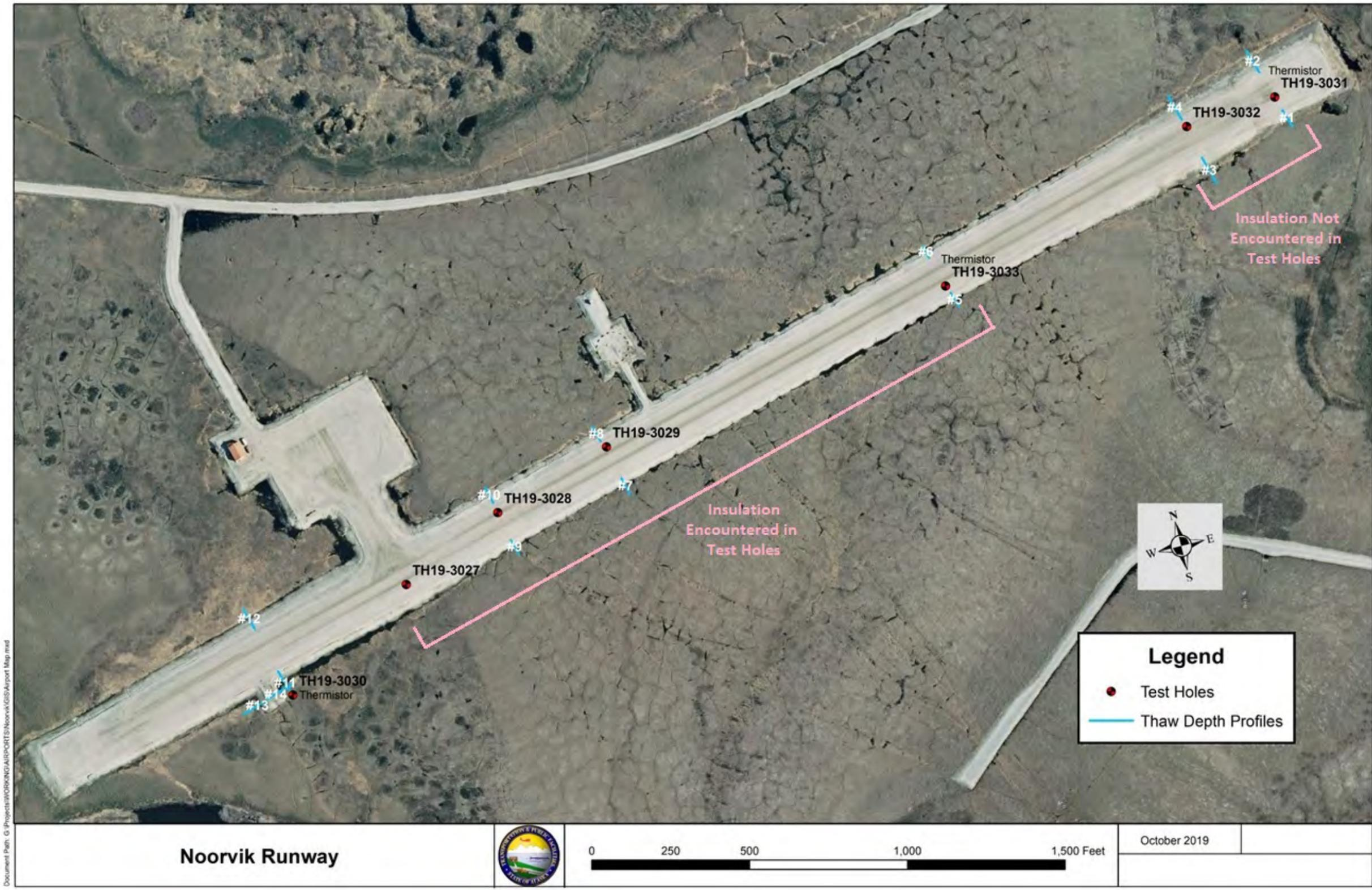
Figure 5. Map of airport test holes, thaw depth profile locations, and occurrence of foam insulation in runway test holes.
