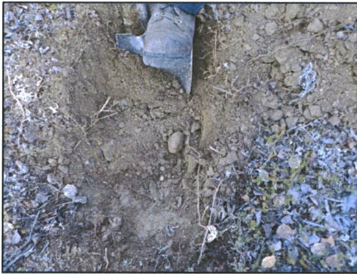
Figure 10. Test Pit 18-118; Silty Gravel with Sand.
