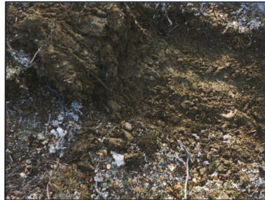
Figure 11. Test Pit 18-122; Silt with Trace Gravel.
