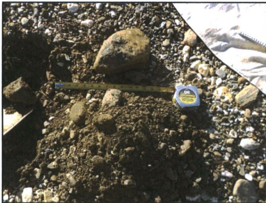
Figure 12. Test Pit 18-124; Poorly-graded Gravel with Silt and Sand.
